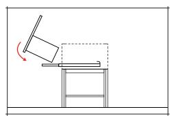
To return the drawer to the unit, fully extend the runners. Tilt the drawer backwards and insert so that the runner intersects the rear of the drawer. Push the runner into the back of the drawer. Locate onto the pins at the front of the runners.
